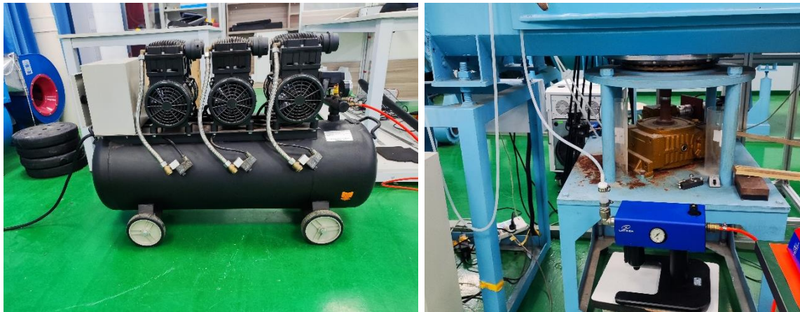
Fig. 2: Compressor and fog generator.
